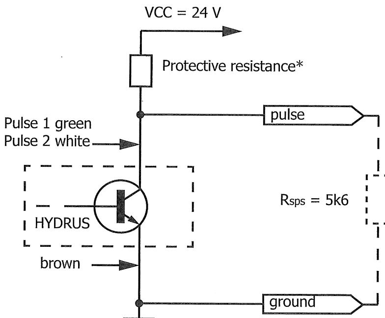
The pulse outputs are open-collector circuits.
